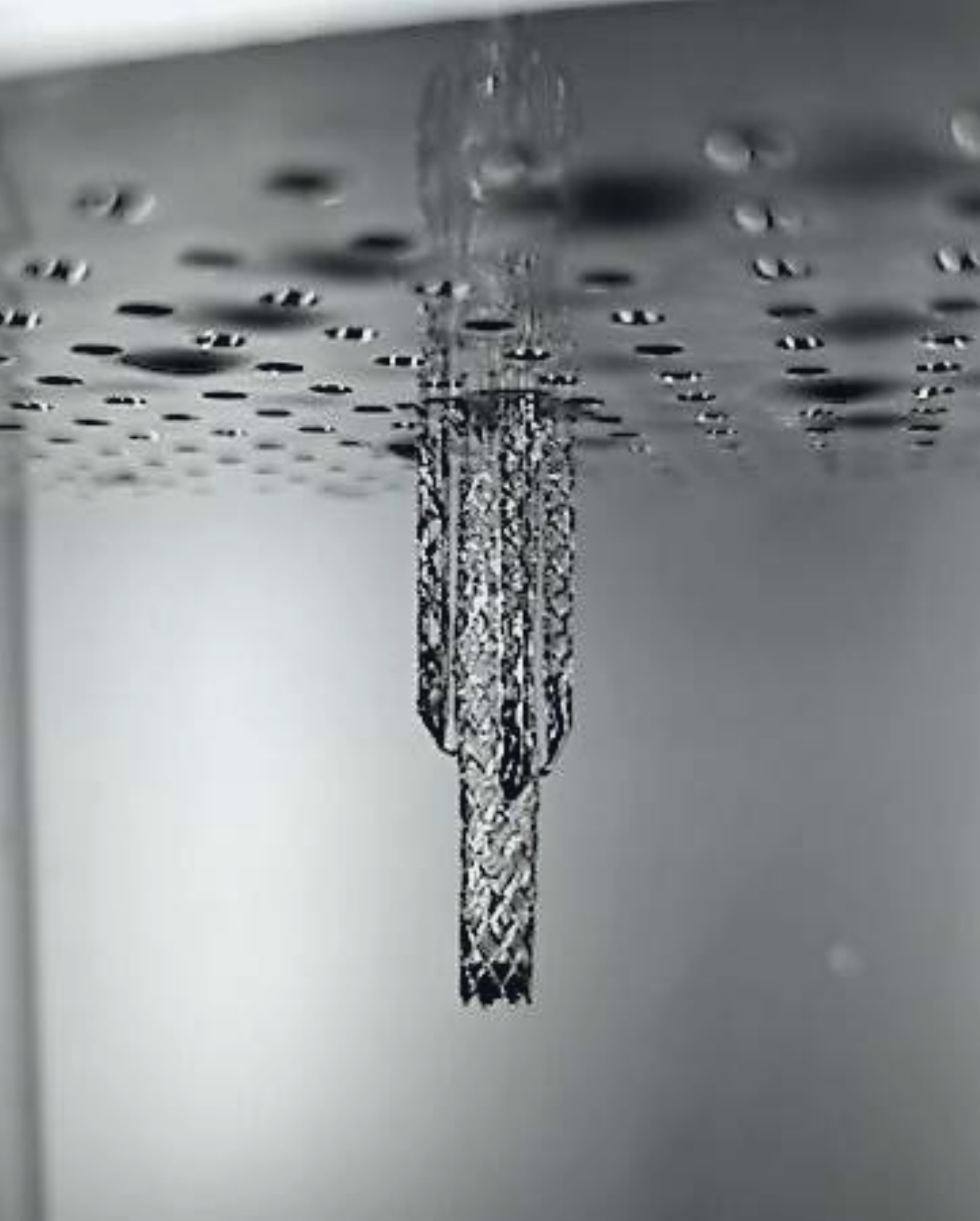
Figure 3 Stent Produced by Lumia.X1
