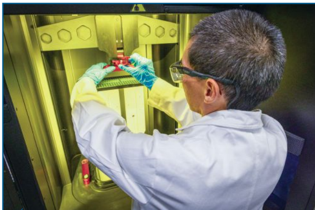
An LSI Solutions team member removes the completed mold from the build plate with ease.
